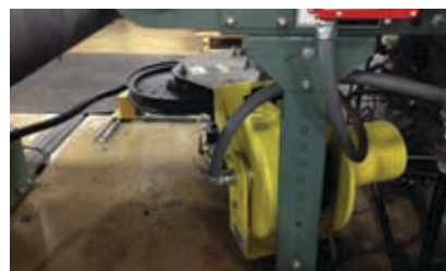
Failing cable due to the “corkscrew” effect
