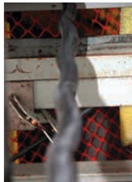
Failing cable due to the “corkscrew” effect
