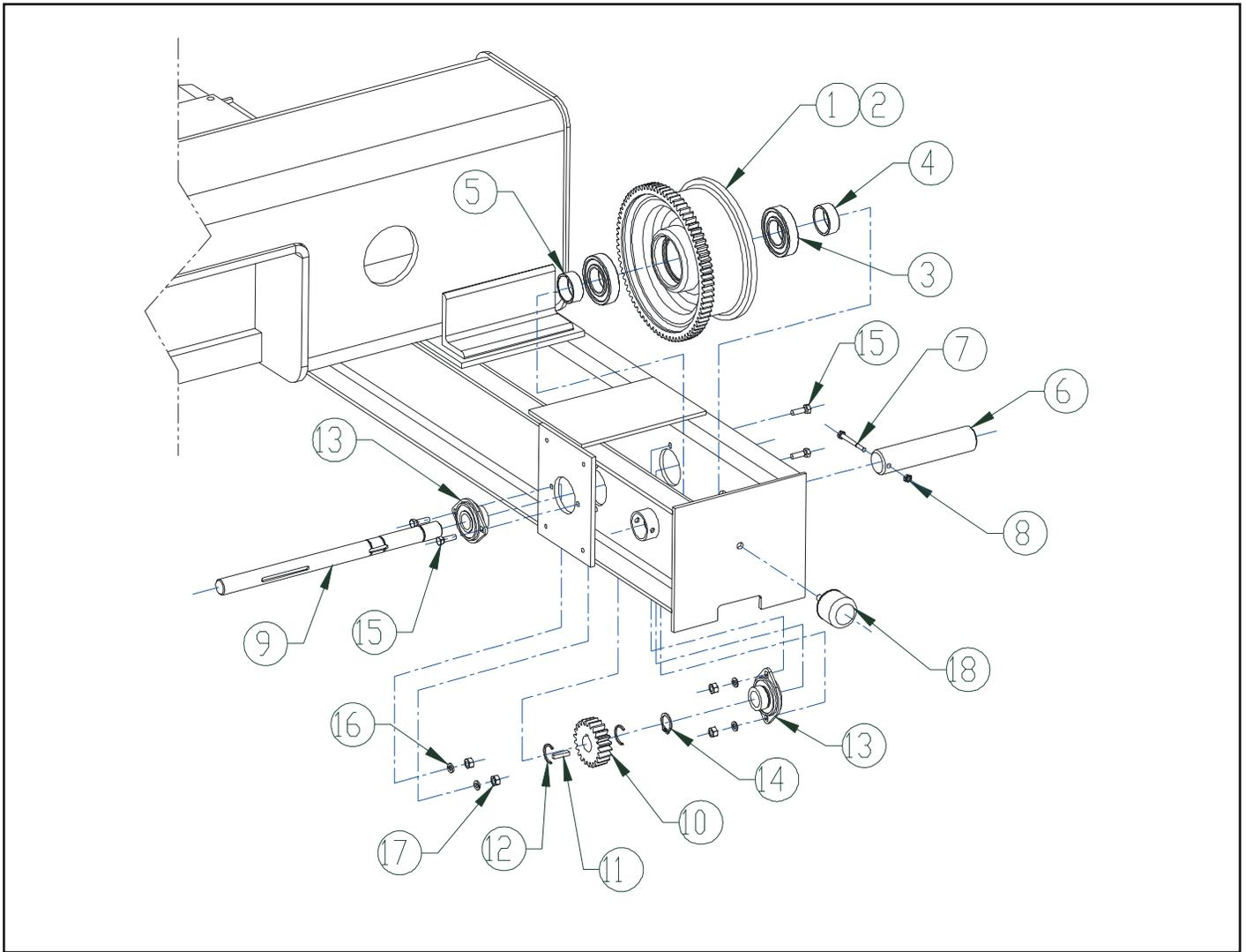
Figure 9-3b. Common Traverse Drive Component
