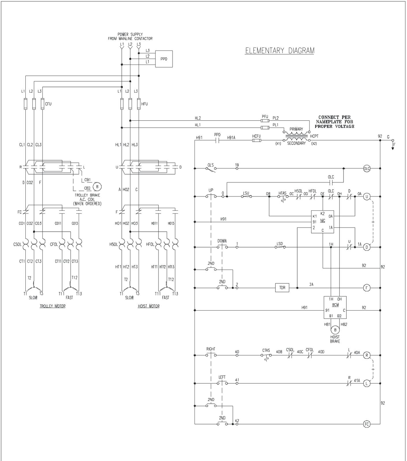
**Figure 8-2. Component Diagram for a Two-Speed Hoist and Trolley with Standard Features**
