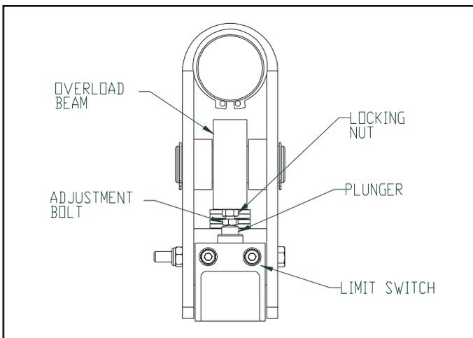
**Figure 7-3a. Over-Capacity Limit Switch ("B" & "C" Frames)**
