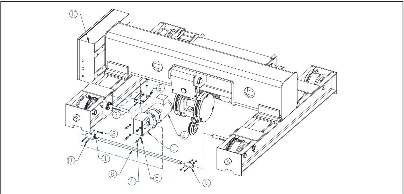
Figure 9-3a. Traverse Drive Component ("B" Frame Shown).
