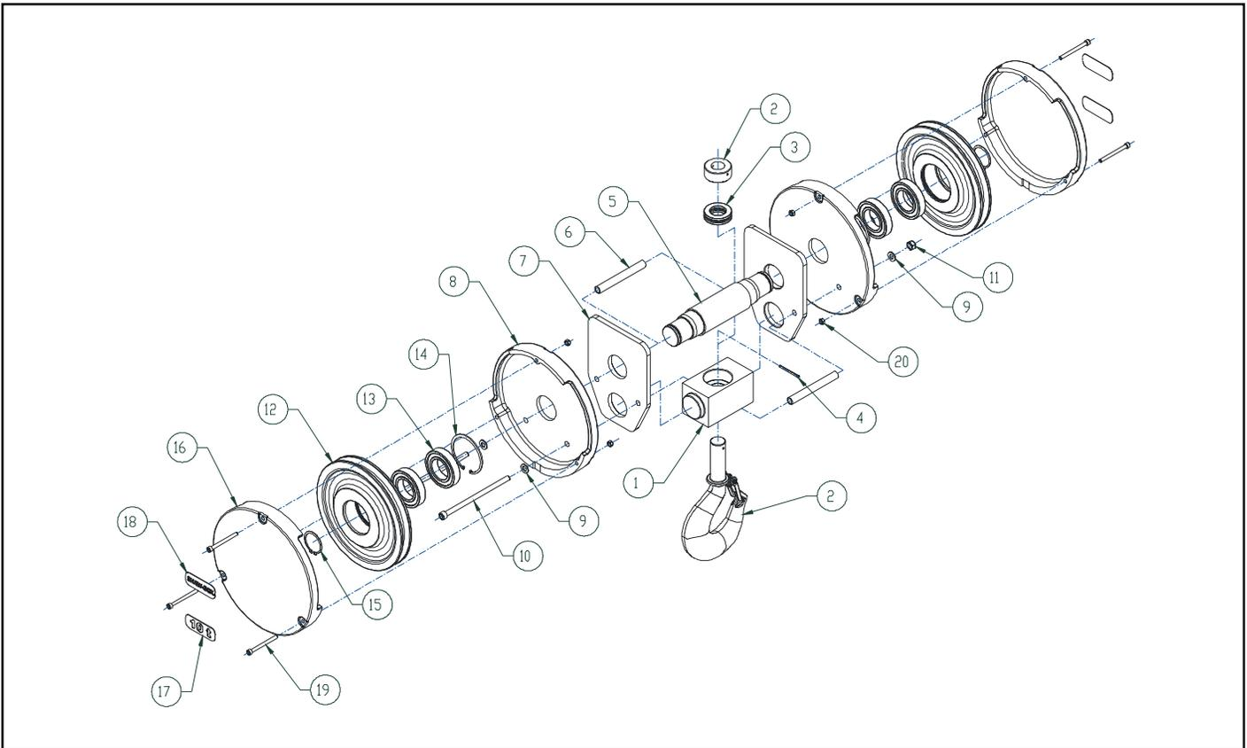
**Figure 9-4a. Lower Block Assembly
