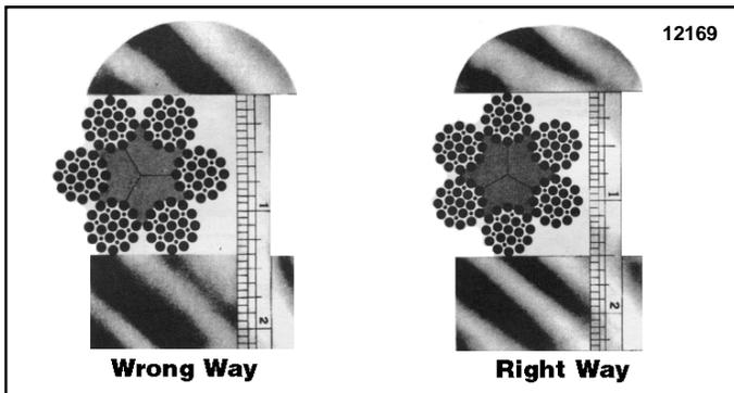
**Figure 5-4. Correct Method of Measuring Rope**
