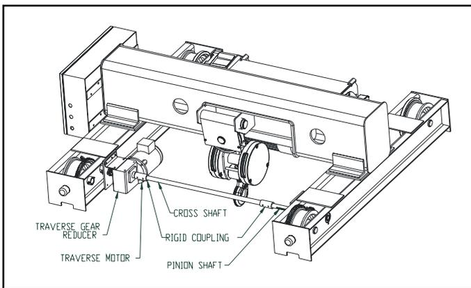
**Figure 5-9. Traverse Drive Arrangement ("B" Frame shown above)**
