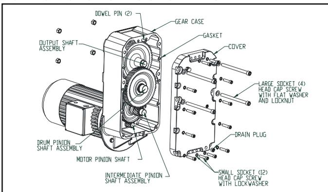
**Figure 5-7. Hoist Gear Case Assembly ("B" & "C" Frame)**
