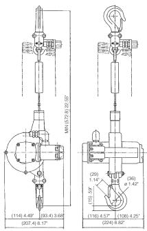
Figure 1 - Hoist Specifications
