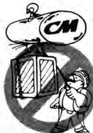
Do not use load chain as a sling. Such usage damages the chain and makes the limit switch setting ineffective.
