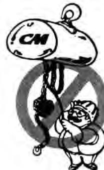
**! WARNING** — DO NOT PULL AT AN ANGLE. BE SURE HOIST AND LOAD ARE IN A STRAIGHT LINE.
