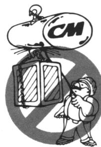
Do not use load chain as a sling. Such usage damages the chain and lower hook.
