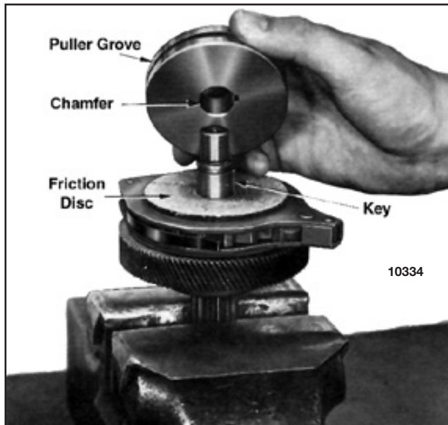
Figure 7-22. View Showing Load Brake Flange Removed
