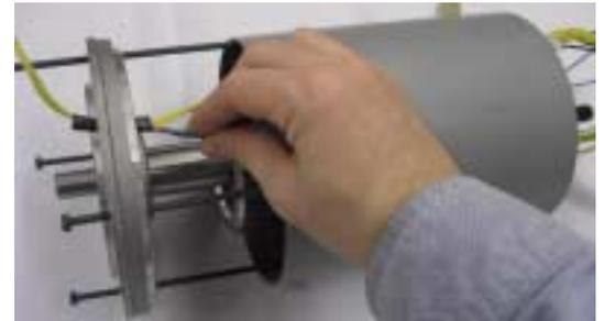
Reinstall motor, pulling wire leads through the gear case wire passage.
